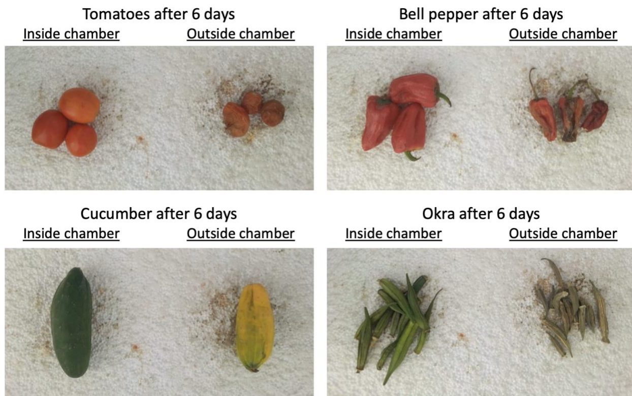
Figure 18: The shelf-life of tomatoes, bell peppers, cucumbers, and okra stored in the forced-air evaporative cooling chamber and outside of the chamber in the shade. The degradation of the samples stored in the shade is clearly visible, while the samples stored in the chamber are still fresh and edible and salable after 6 days.
