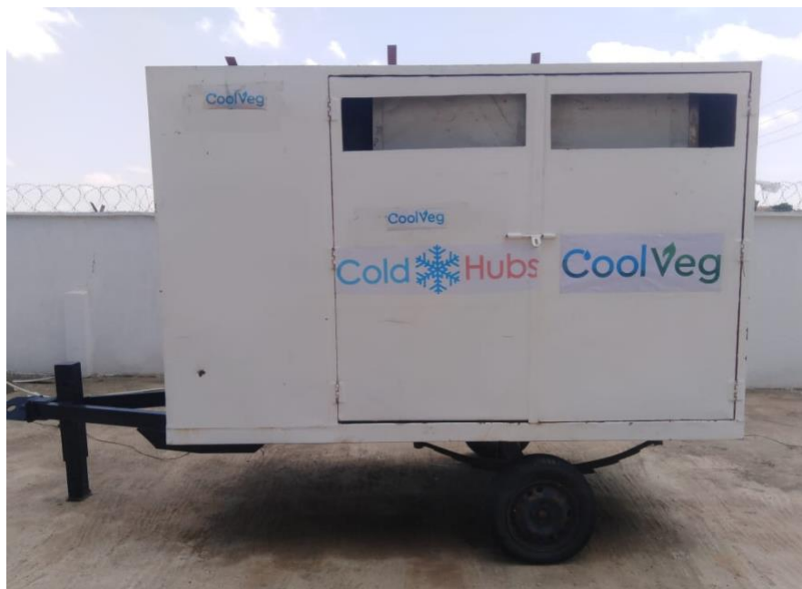
Figure 7: A trailer-based mobile forced-air evaporative cooling chamber, with the steel exterior side doors visible. The insulation chamber is housed inside the exterior metal shell and can be seen through the exhaust vents at the top of the side doors.
