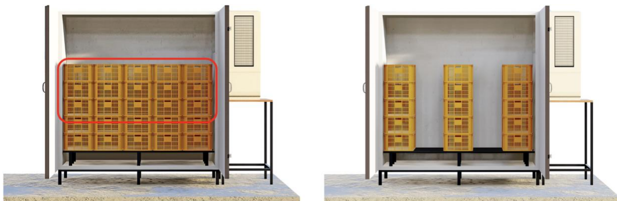
Figure 12: Left: the crate configuration for the “High fan (15)” and “Low fan (15)” tests, where only the top three rows of crates are considered, represent the cooling of 15 crates. Right: the crate configuration for the “AC (15)” tests, where two stacks of crates were removed to allow for airflow between the remaining stack of crates. This type of configuration is commonly used in cold rooms.
