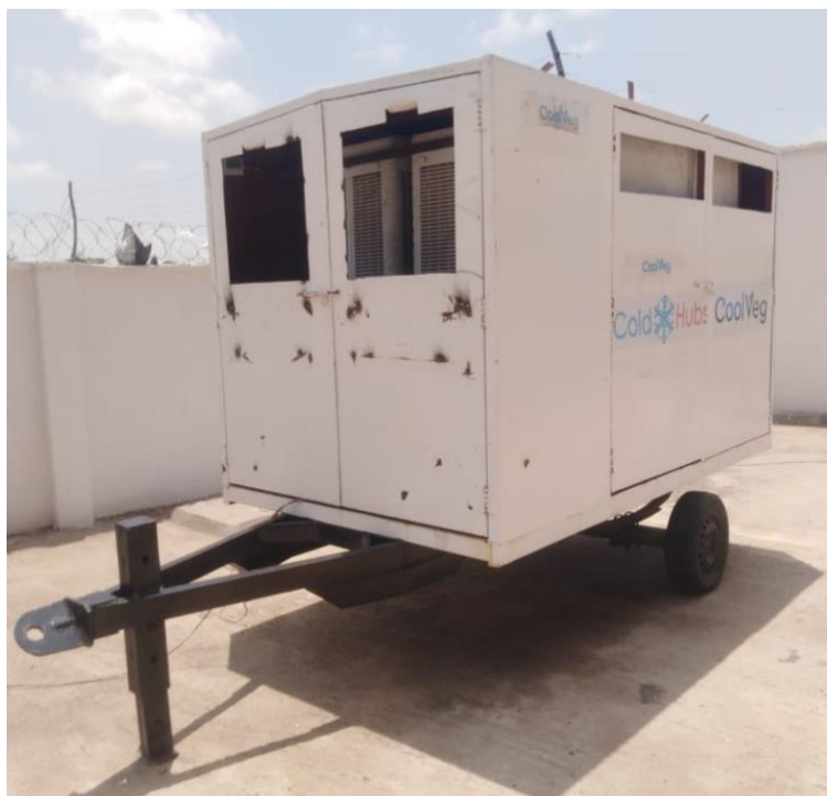
Figure 8: A trailer-based mobile forced-air evaporative cooling chamber with the front and right side visible. Two evaporative coolers are located in an enclosed front compartment, visible through the square windows in the front of the chamber.
