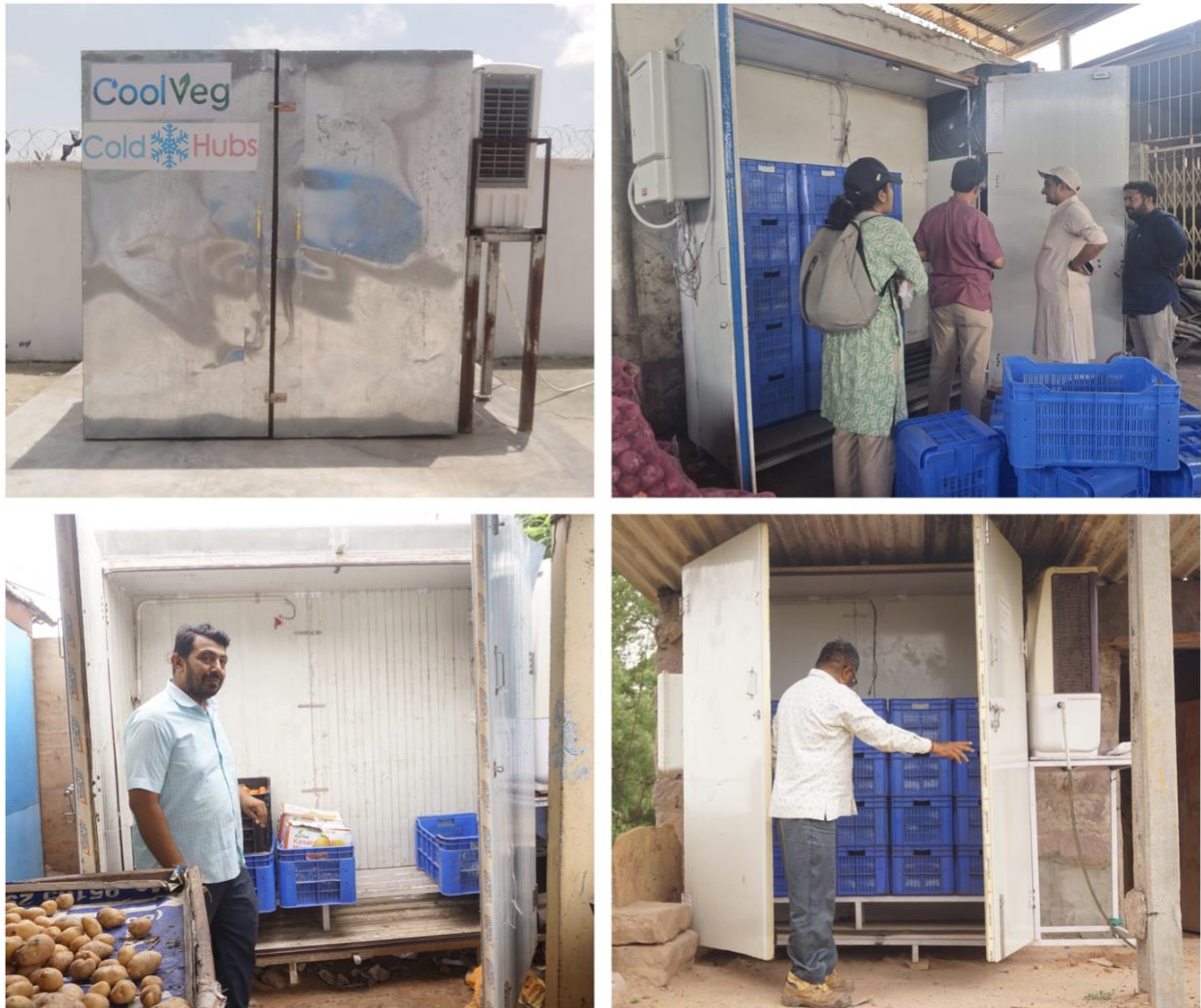
Top left: Portable cooling chamber with a storage capacity of 25 crates in Zaria, Kaduna, Nigeria; Top right: Portable cooling chamber with a storage capacity of 25 crates in Bhuj, Gujarat, India; Bottom left: Portable cooling chamber with a storage capacity of 15 crates in Bhuj, Gujarat, India; Bottom right: Portable cooling chamber with a storage capacity of 20 crates in Bhuj, Gujarat, India.
