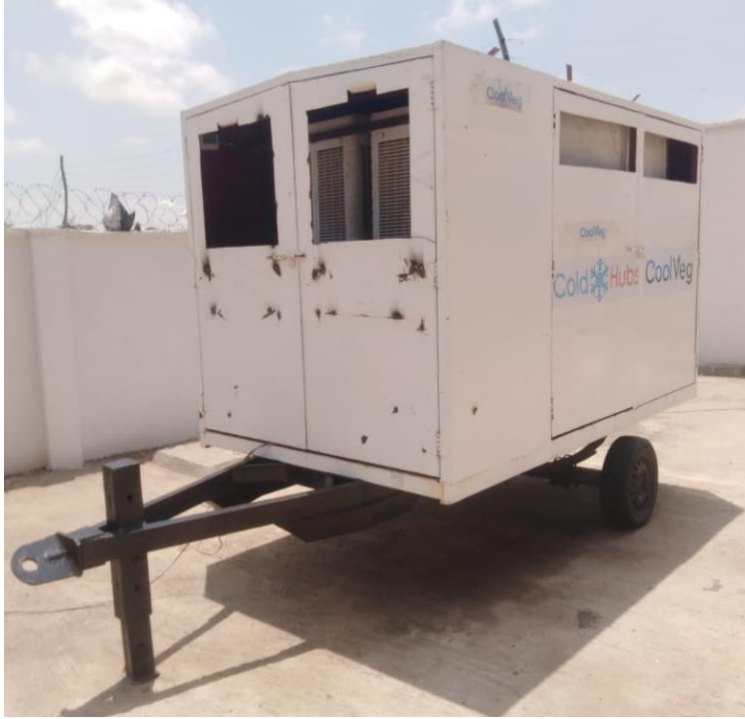
Figure 2: A trailer-based mobile forced-air evaporative cooling chamber with the front and right side visible. Two evaporative coolers are located in an enclosed front compartment, visible through the square windows in the front of the chamber.
