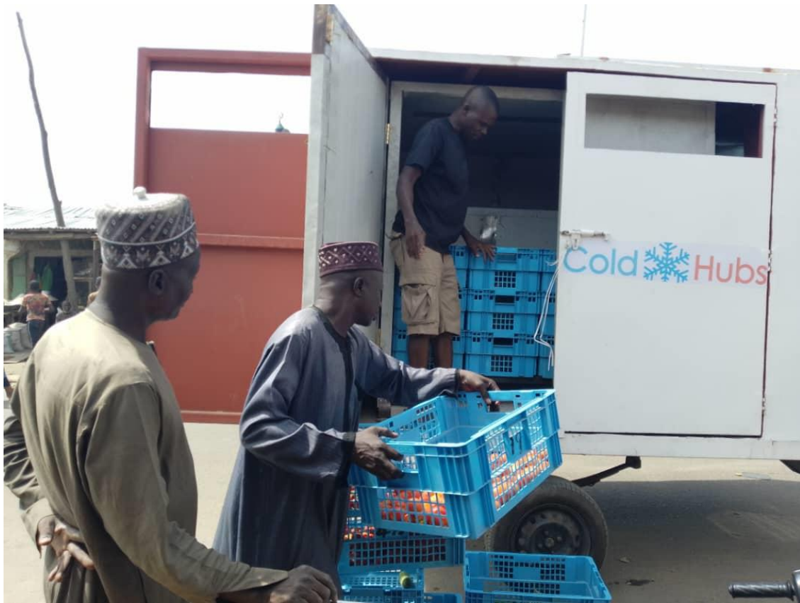
Figure 3: Vendors loading produce into a trailer-based mobile forced-air evaporative cooling chamber. The chamber has a storage capacity of 32 crates, or 640 kgs of produce.
