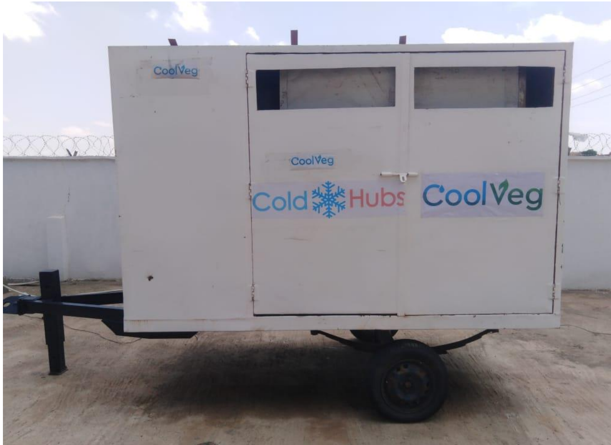
Figure 1: A trailer-based mobile forced-air evaporative cooling chamber, with the steel exterior side doors visible. The insulation chamber is housed inside the exterior metal shell and can be seen through the exhaust vents at the top of the side doors.
